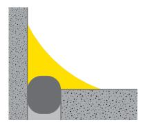
Fillet joints are being used between two intersecting elements, for example sealing the window frame perimeters from outside. To assure the sealant adhesion, the contact surface between the sealant and the surface needs to be at least 6 mm.
