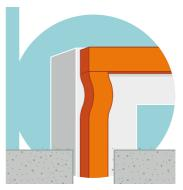
Position horizontal band first to terminate the vertical band position. Provide 1 cm of seal over-length on the vertical bands. Do not rotate the tape around the corners.
