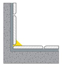
Fillet joints are being used for practically immovable connections (inner corners of walls, the connections of sinks and toilets). The triangular shape of the sealant helps to avoid the water accumulation on sealant's surface.
