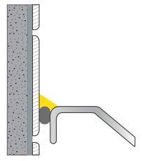
Before sealing the joint between the wall and bathtub, the bath should be supported correctly to avoid unwanted movements during exploitation. With wider joints, backer rod should be used.
