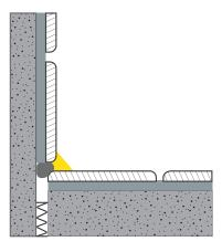
When sealing joints with greater deformations (e.g. joints between the wall and floating floor), suitable backing material, such as closed cell PE backer rod, should be used to avoid three-sided adhesion and give the sealant the correct form.
