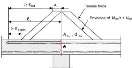
**Figure 2:** Overlap joint in foundation of a column or wall where the rebars are stressed in tension.
