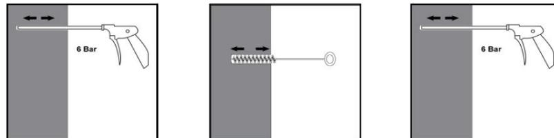
Blow 2 times from the back of the hole (if needed with a nozzle extension) over the whole length with oil-free compressed air (min. 6 bar at  $6\text{ m}^3/\text{h}$ ). Brush 2 times with the specified brush size (see Table 6) by inserting the steel brush to the back of the hole (if needed with an extension) in a twisting motion and removing it.
