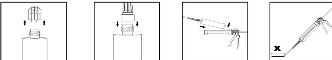
Remove the threaded cap from the cartridge. Tightly attach the mixing nozzle. Do not modify the mixer in any way. Make sure the mixing element is inside the mixer. Use only the supplied mixer. Insert the cartridge into the dispenser gun. Discard the initial trigger pulls of adhesive. Discard the first 12ml of resin. Please note that after every subsequent mixer change, an initial 12ml of resin should be extruded to waste to continue with even mixing.
